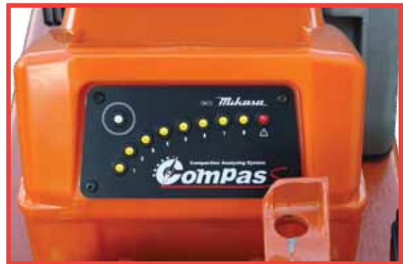
LED lights guide operator as soil density increases
