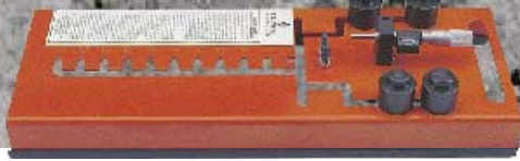
Blade Measuring Gauge Dial or Digital available: indicates the wear on a diamond blade. Great for measuring rental blades.
