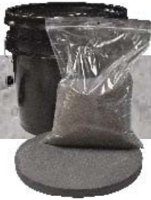
Bit Sharpening Pot Plastic bucket that includes a cast iron plate and #60 aluminum oxide sand for sharpening dull core bits. The sand acts as an abrasive to expose the diamonds in the segments.
