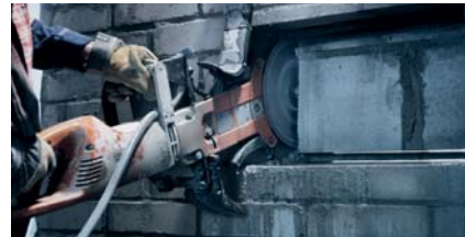
Efficient electric cutter with convenient method for cutting up to 16" deep.
