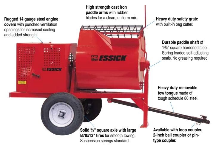
Essick 12 cubic foot plaster/mortar mixers are available with mechanical drives.
