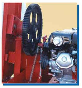
Double V-belt/gear drive. Idler wheel provides easy, positive engagement. Allows larger, heavier mixes. Cast-steel pulleys increase durability.
