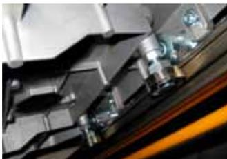
Precise fore/aft tracking is assured by the unique locking ball bearing roller assembly. This unique design ensures that no axial play can be introduced to the conveyor cart. Material will travel straight and true into the cutting diamond blade.
