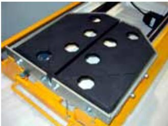
The die-cast aluminum conveyor cart with heavy NBR rubber injected molded top pad ensures the flat/secure orientation of the material. The well designed drain holes and accurate back ruler fence assist the operator in cutting efficiency.
